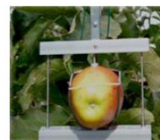
Type DF Fruit Dendrometer. Suitable for diameter < 11 cm
