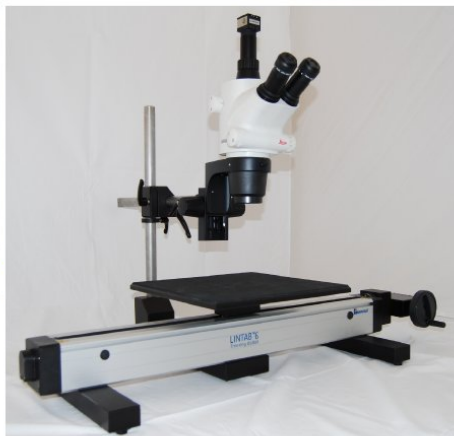
LINTAB™ 6th generation since 1990: robust, precise, durable, high resolution (1/100 or 1/1000mm).
