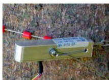
Type DC1 Circumference Dendrometer 1. Suitable for diameter 5-30 cm. No injury to plants
