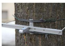
Type DD-L Diameter Dendrometer Large. Suitable for diameter 3-30 cm. No injury to plants
