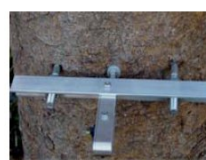
Type DR Radius Dendrometer. Suitable for diameter > 8 cm
