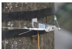
Type DC2 and DC3 Circumference Dendrometer 2 and 3. Improved version of DC1, suitable for diameter > 5 cm. The automatic adjustment of pressure to the tree enhances sensitivity and enables the comparison of measuring data of different tree size. No injury to plants
